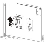
When the **System Enable** switch is in the ON position, the Startup screen appears on the display interface of the Symmetra PX UPS.
